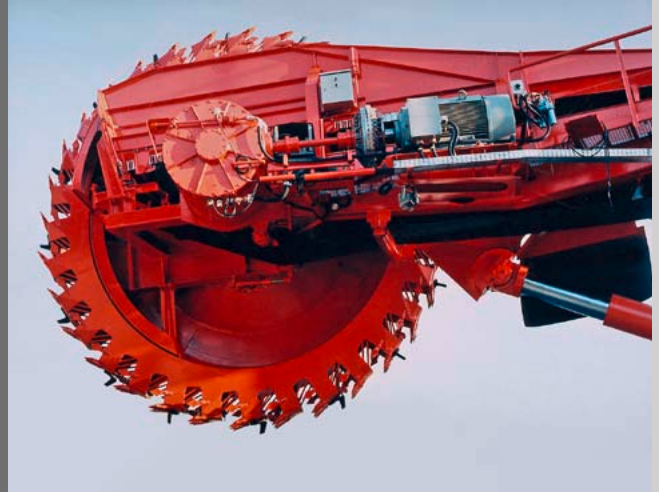
Fig. 26: Voith Turbo fluid coupling in a bucket-wheel excavator drive
