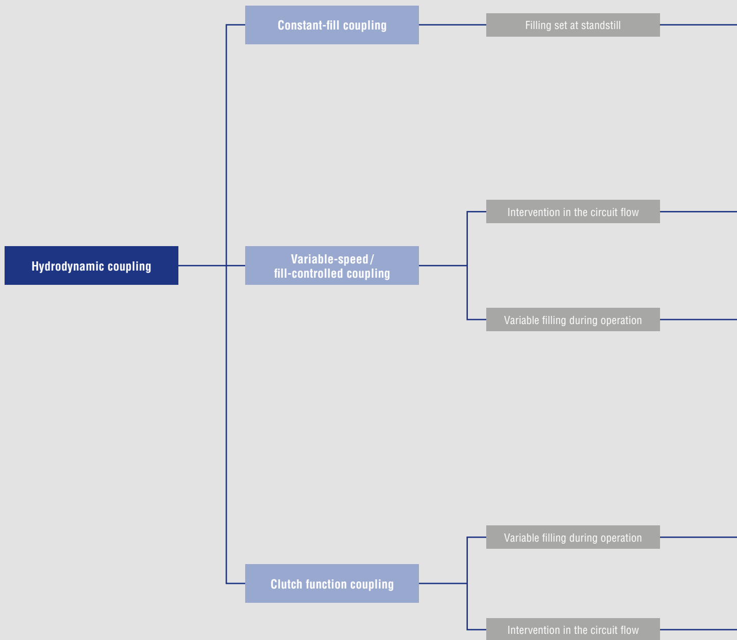
Fig. 35: Structure of the designs of hydrodynamic couplings according to directive VDI 2153 – according to the terminology of the shaft couplings
