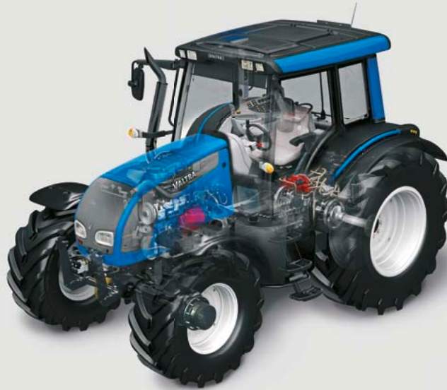
Fig. 30: Tractor with hydrodynamic constant-fill coupling in the drive chain
