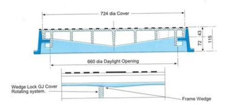
Any EMBLEM such as Telecom is optional as and when required and ordered. Rotate Cover Anti-Clockwise to Lock and Clockwise to Cut out stopper in Frame to Lift out.
