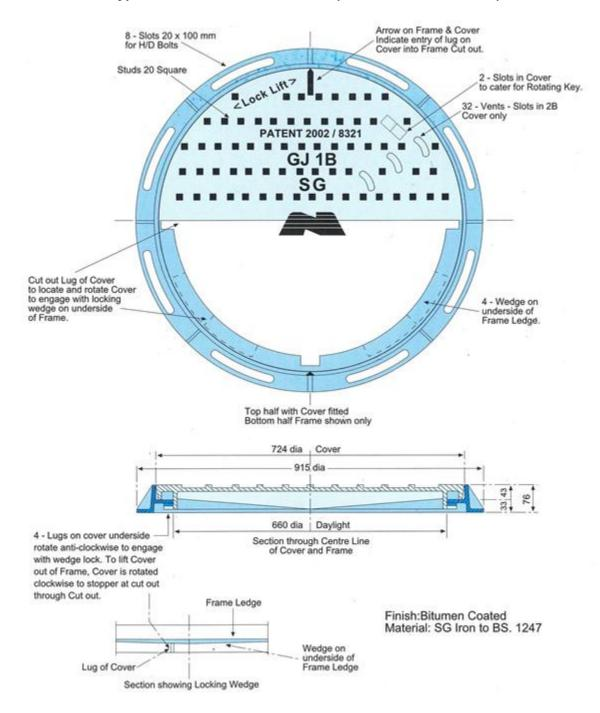
TYPE GJ 1B (With Vents - Slots in Cover) Round Frame Medium Duty - Work Load - 30 Mt Minimum For - FOOTWAY.
