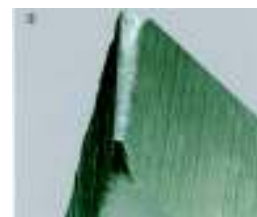
3. Excessive strain by improper breaking in leads to micro breakages of the cutting edge
