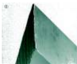
1. New cutting edge with very small edge radius
