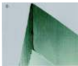
2. Proper breaking in of the bandsaw blade creates an optimal rounded cutting edge
