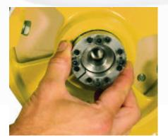
No internal bearings that can be damaged when the medium enters due to hose breakage, resulting in complete pump failure
